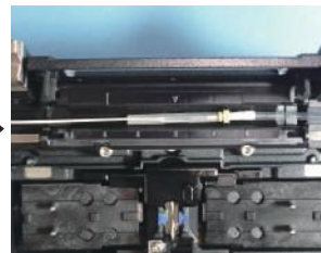
3. protection sleeve shrinking
