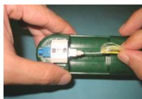
3. Set connector and cord onto assembly tool and insert fiber to connector
