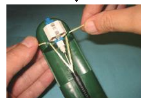
6. Tighten boot, remove connector from assembly tool and trim aramid yarn
