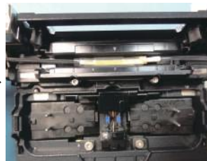
3. protection sleeve shrinking
